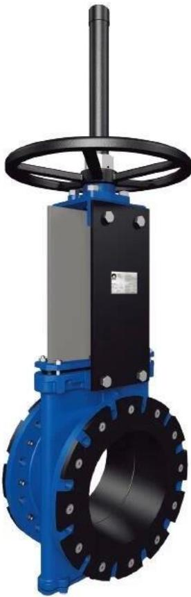
Bidirectional lug knife gate valve. Wide design "Monoblock" one-piece cast iron body. Stainless steel gate. Two body-bolted rubber sleeves. Provides high flow rates with low pressure drop.
