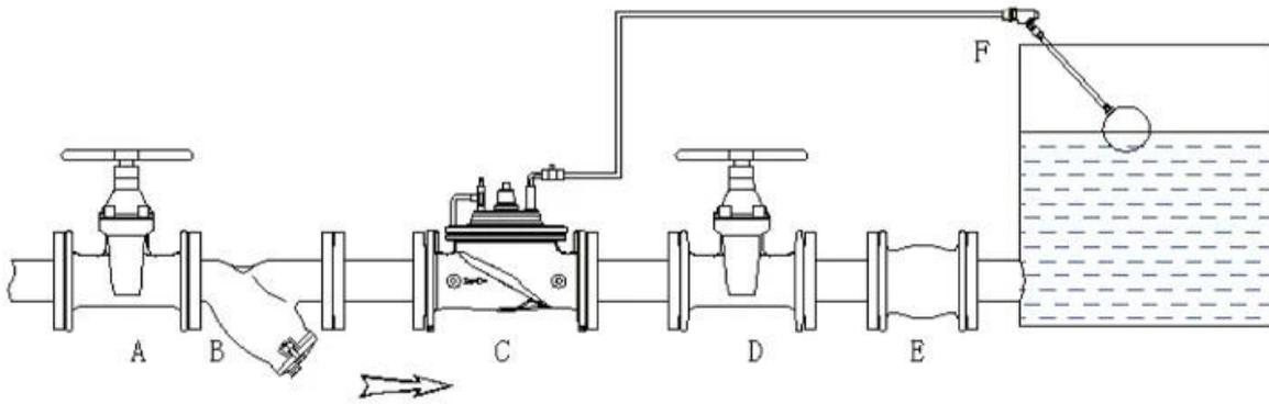
A. Shut Off Valve B. Y C. Float Control Valve D. Shut Off Valve
