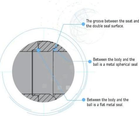
The groove between the seat and the double seal surface.
