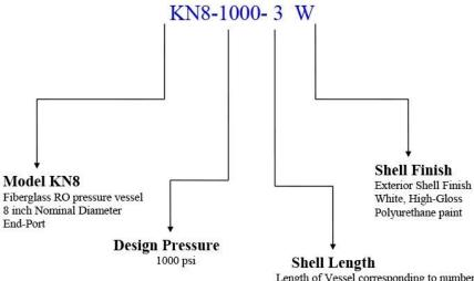
Length of Vessel corresponding to number Of 40" elements that can be contained
