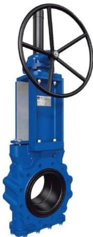
Bidirectional high pressure lug-wafer-design knife gate valve. "Monoblock" one-piece cast iron body. Stainless steel gate. Two rubber sleeves. Provides high flow rates with low pressure drop.
