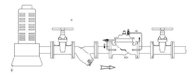
The 745X dual-chamber multi-function pump control valve is installed at the pump outlet to prevent and eliminate the damage of water hammer to the pipeline system/pump when the pump is turned on/off $\Box$
