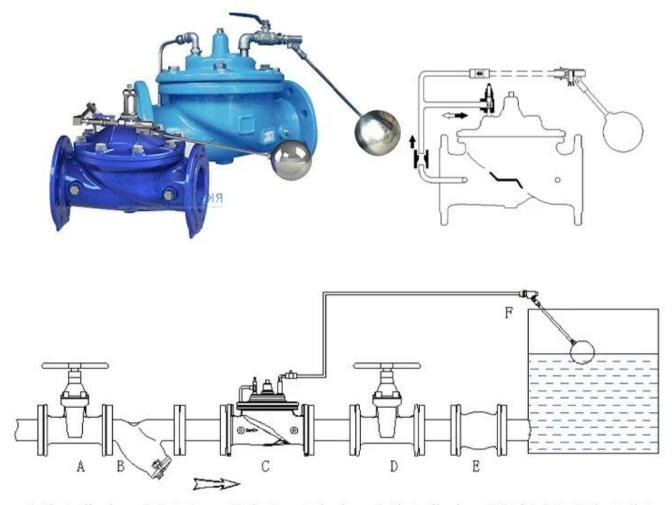
A. Shut off valve B. Y strainer C. Float control valve D. Shut off valve E. Soft joint F. Float pilot
