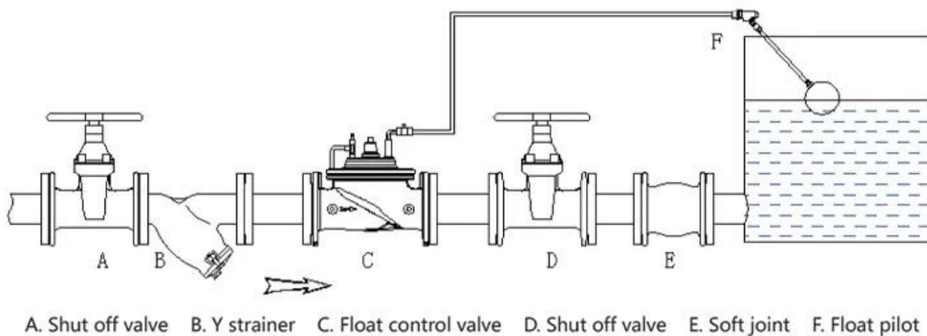
A. Shut off valve B. Y strainer C. Float control valve D. Shut off valve E. Soft joint F. Float pilot
