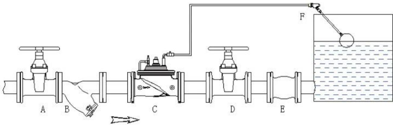
A. Inlet shut-off valve B. Y-filter C. Float control valve D. Outlet shut-off valve
