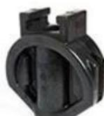
**Male guiding system with composite sliding skate** reduces the wear of the wedge against the body, allowing a smooth functionality and a longer life time of the valve.
