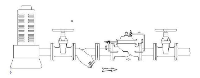
The 745X dual-chamber multi-function pump control valve is installed at the pump outlet to prevent and eliminate the damage of water hammer to the pipeline system/pump when the pump is turned on/off  $\square$
